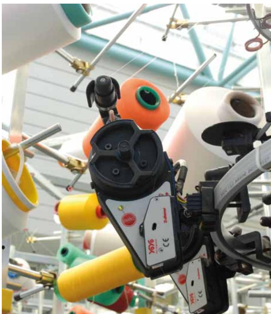
**YOYO** device performs the control of yarn feeding in the textile machines (large diameter, seamless, hosiery and flat knitting machines) using a programmed weight. The control system, based on a high performance sensor and motor, can be programmed to set up and maintain the yarn with different tensions, according to the specific manufacturing and to the different types of yarn. **YOYO** has been studied to completely integra-
