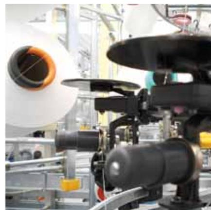
The **SPYDER** is a yarn breakage device that detects the yarn feeding into the textile machines (large diameter, seamless and hosiery knitting machines).
